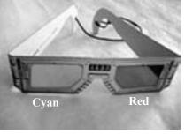
Two of these 3D glasses are crossed as shown. Where the red and cyan filters overlap, the glasses appear black.
